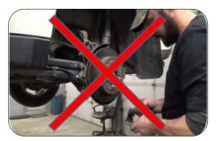
Do not work on brake pads without a mask (as a minimum) to avoid exposure to asbestos.
