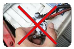
Do not handle batteries or clean the terminals without gloves. Remember, batteries contain acid and baking soda is used to clean terminals. Both are toxic and corrosive.
