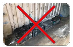
Do not store used batteries in an area exposed to heat, without proper ventilation and without draining the acid first (batteries will corrode and leak contaminants into the environment).
