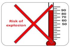
Never expose airbags to excess heat (over 90 degrees Celsius) due to the risk of explosion.
