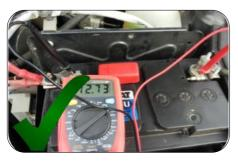
Ensure batteries are well maintained: clean battery terminals, maintain electrolyte level and verify the voltage with a multimeter.
