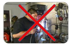
Do not weld without the proper equipment. Welding fumes are toxic and long-term exposure to the welding damages the eyes.
