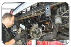
Do not handle brake pads, clutch parts, or gaskets without protective equipment, as they may contain asbestos. It is not possible to distinguish if a component contains asbestos just by looking at it.
