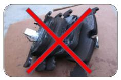
Do not store new or used brake pads without protection or clear labelling. Remember, brake pads might contain and release asbestos fibres. Do not dispose of them on unprotected soil or waterways.
