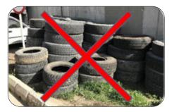
Do not store tyres exposed to the sun or rain, without protection, in order to avoid cracking of new tyres and mosquito breeding.
