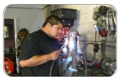
Do not weld without the proper equipment. Welding fumes are toxic and long-term exposure to the welding arc damages eyes.
