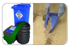
In case of a toxic chemical spill (e.g. brake fluids and coolants), use a spill kit or absorbent material to contain the spill and clean the area. Protective equipment should be worn.
