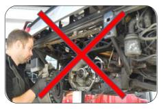
Do not handle brake pads as if they were asbestos-free. It is not possible to distinguish if a component has asbestos just by looking at it.
