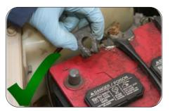
Use personal protective equipment (safety boots, goggles, gloves) when filling/replacing battery acid and cleaning terminals with baking soda.
