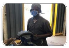
Use a mask or a respirator to prevent dust and asbestos inhalation while working on brake pads and other spare parts. Avoid exposure to asbestos dust, it is highly toxic.
