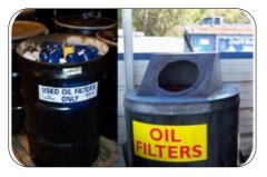
Store hazardous waste (asbestos, electronic waste, spent oil, etc.) in proper containers and designated areas. Avoid exposure to toxic substances.
