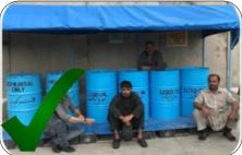
Separate spent oil and lubricants by type. Store them in closed, labelled containers on a pallet or hard surface. Spent oil and lubricants should be disposed of by an authorized contractor or local recycler.
