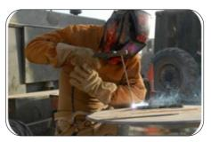
Use an appropriate full face mask, safety boots, gloves and overalls when welding. Protect yourself from fire risk and your eyes from the welding arc.
