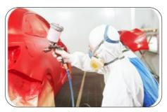
Use PVC gloves, safety boots, protective overalls with hood and an air-purifying respirator when painting. Avoid exposure to toxic fumes.
