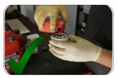
Ensure filters are correctly installed in line with the manufacturer's recommendations to maximize the lifespan of each filter and minimize waste.
