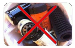
Do not mix metallic filters with paper or cardboard filters. Remember that metallic filters can be recycled if properly drained, and paper filters could be used as fuel in facilities such as cement factories.
