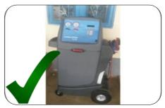
Whenever possible, prioritize refrigerant recovery using appropriate equipment, rather than venting gas into the atmosphere. Ensure proper disposal/ exchange of empty cylinders by authorized contractors.
