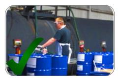
Always use appropriate personal protective equipment (safety boots, goggles, gloves) when handling spent oil and lubricants.
