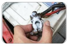
Do not handle batteries, battery acid or clean the terminals without gloves. Both acid and caustic soda are toxic and corrosive.
