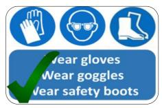
Use appropriate tools and protective equipment (safety boots, goggles, gloves) when handling used drums, regardless of the drum type and what it previously contained.
