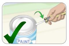
When opening tins of paint, use a tool to avoid damaging the tin. This prevents waste from the paint from drying out.
