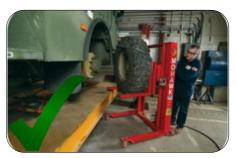
Use appropriate personal protective equipment (safety boots, goggles, gloves) when handling tyres, especially heavy duty tyres.
