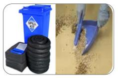
In case of a chemical or fuel spill, use a spill kit or an absorbent material to contain the spill and clean the area. Use protective equipment (safety boots, goggles, gloves) when performing the cleanup.
